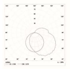
Correlated color temperature: 3000-6000 kelvin Rated median useful life: 50000h L70 at 25°C Luminaire input power: 5 w
